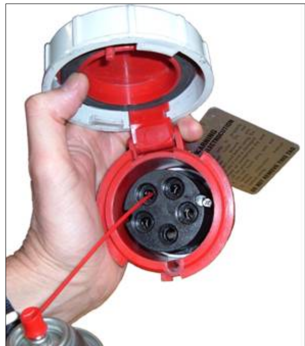
Figure 14: Lubricate the receptacle.
