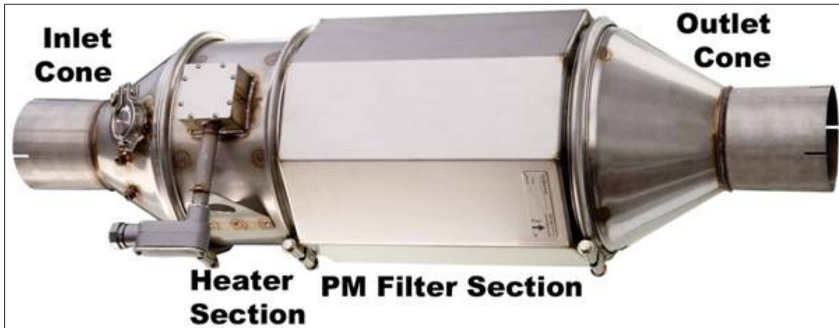
Figure 2: PM Filter Assembly.
