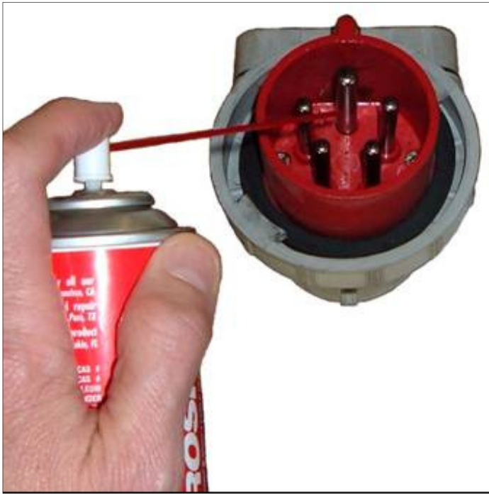
Figure 13: Lubricate the plug.
