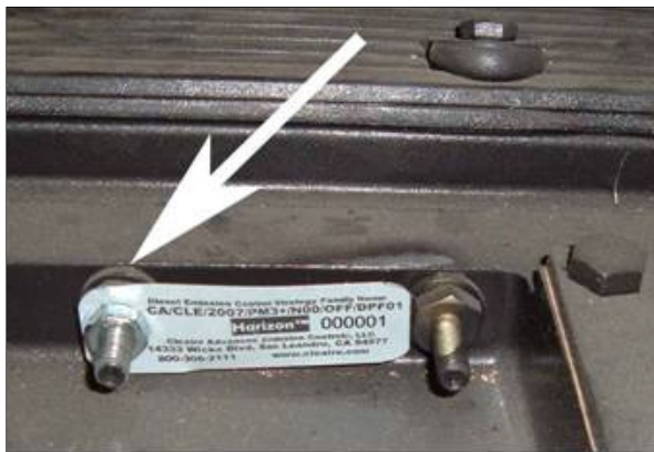
Figure 7: Example of CARB-verification label for Horizon installed on engine.
