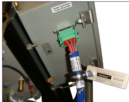
Figure 8: CARB-verification label attached to wiring harness at Horizon Controls Box.
