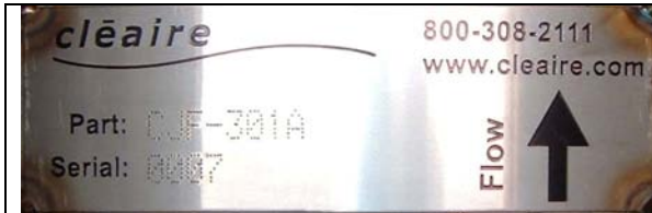
Figure 7: MDPF part tag and flow arrow.
