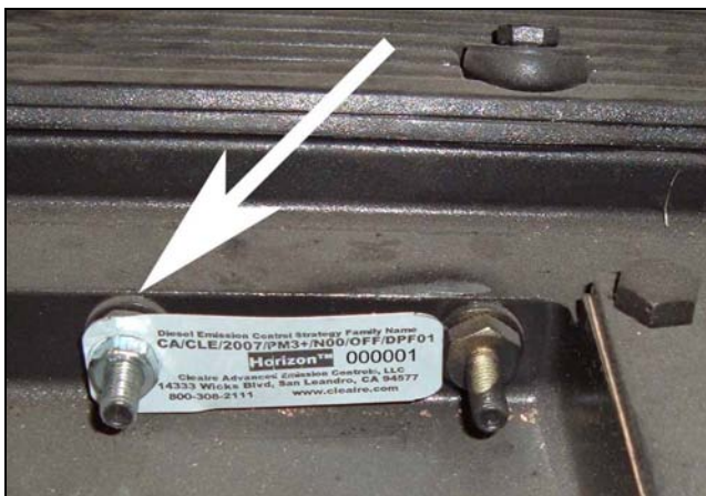
Figure 3: Example of CARB-verification label installed on engine. (Example is from a Horizon system.)
