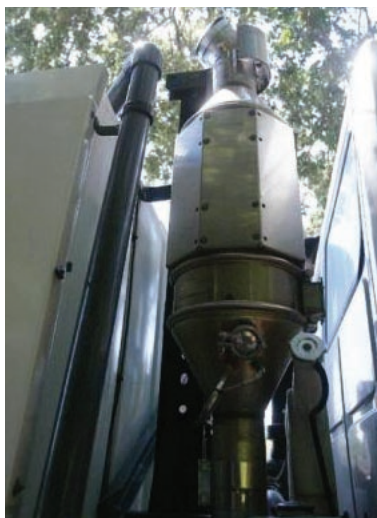
A $12,000 filter installed on the city's diesel vehicles is expected to lead to cleaner air.
